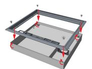
8. Secure the lid frame to its position by fastening the screws on all four sides
