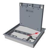
9. Place the lid's dome hinge on one of the frame and push other side of lid till the hinge slots into its position
