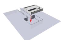
Take the lid and put aside for later. Place the casing into the pre cut screed as per the floor plan. Ensure the casing sits as even as possible with the floor level
