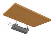
Define the Profilebox Sub's location and ensure that there is a minimum clearance of 15mm each side between the Profilebox Sub and the table edge or neighbouring obstacles.
