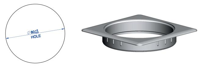
The outer ring of the cable entry is fitted with 12 lamellas.
