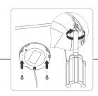
Tighten the unit by screwing the 3 screws to ensure unit fits to the grommet hole
