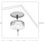
Insert the unit to the grommet hole from the bottom
