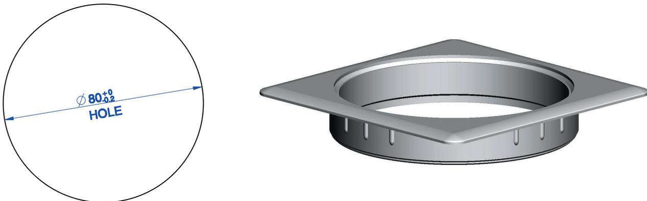
The outer ring of the cable entry is fitted with 12 lamellas. These lamellas provide for a secure grip and prevent, that the ring rotates in the tabletop. The outer dimensions measured on the lamellas is 80.2 mm.
