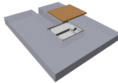
5. Put on the protective hard carton cover. Complete the casting work
