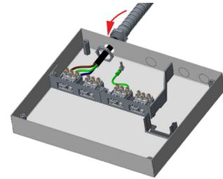
3. Remove the knockouts to install electrical wiring and data cables accordingly. Ensure the earth wire is connected to the terminal
