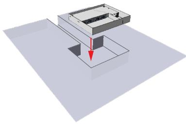
1. Take the lid and put aside for later. Place the casing into the pre cut screed as per the floor plan. Ensure the casing sits as even as possible with the floor level
