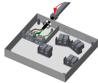
3. Remove the knockouts to install electrical wiring and data cables accordingly. Ensure the earth wire is connected to the terminal
