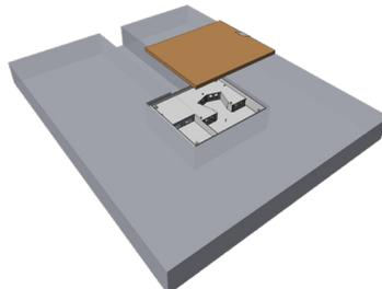
5. Put on the protective hard carton cover. Complete the casting work
