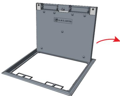
7. Push the lid beyond the opening angle of 109 degrees to detach the lid from the frame
